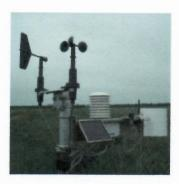
Meteorological station will provide accurate information to the ICC offices related temperature, humidity, solar radiation, wind speed, pressure, precipitation, evaporation, diseases outbreaks for different crops. Based on this information ICCs will provide information related pest and irrigation to the Zrda targeted farmers by SMS
