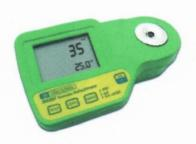
Digital refractometers provide a direct read-out of the soluble solids content. This test is typically used on sub-samples of randomly selected fruit to establish a correlation between fruit size, appearance, and maturity.
