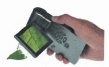
Digital microscope will allow extension agents to identify diseases and insects in the field. If identification of pests will not be possible on the field extension agent can take pictures and make office work.
