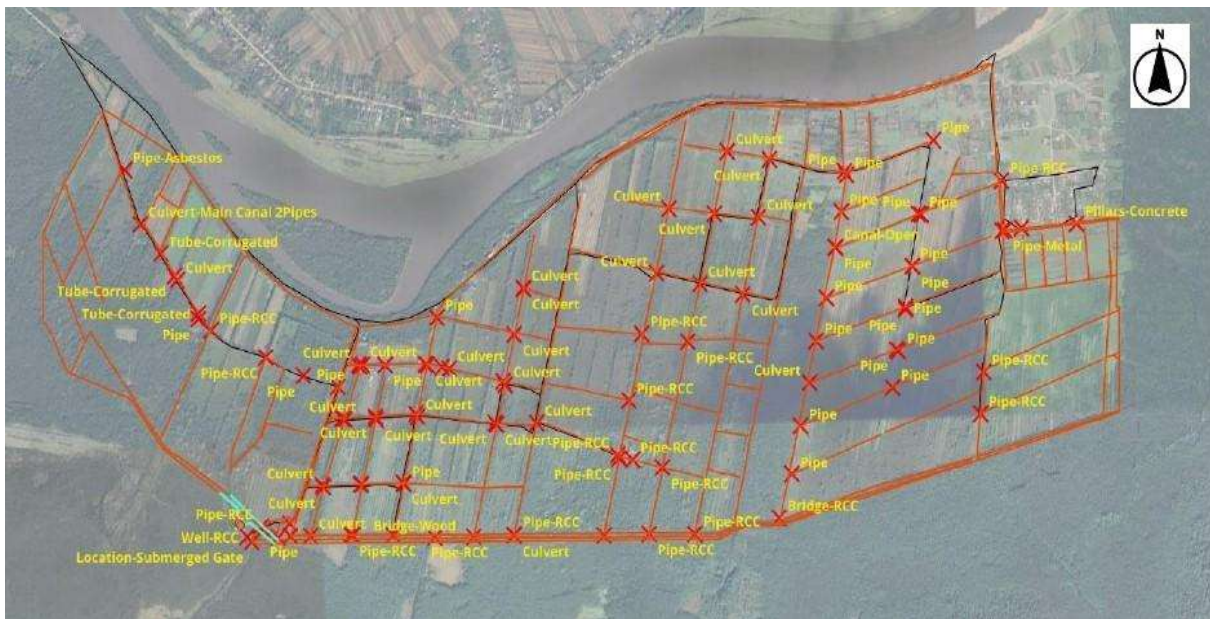
Figure 3: Existing Structures in the SMDS
