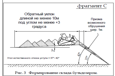
Fig. 5. Formation of the slag by bulldozer.
