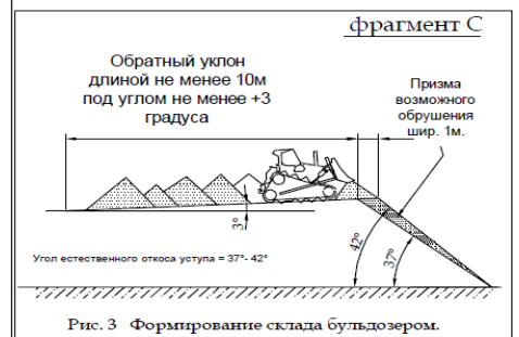
Fig. 3. Formation of the slag by bulldozer.
