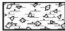
Andesite-basalts crushed stones and boulders with hard plastic consistency loam filler up to 35%.
