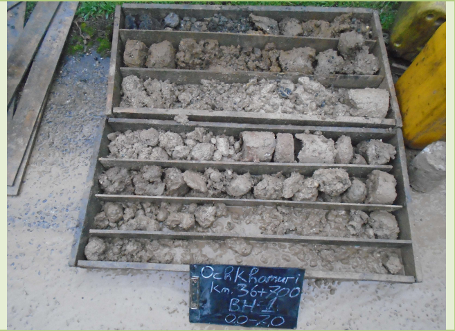
Photo 2. Bridge, BH 1, 0.0-7.0m
